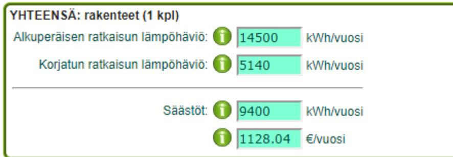
Figure 14: Calculation of saving potential for additional insulation
