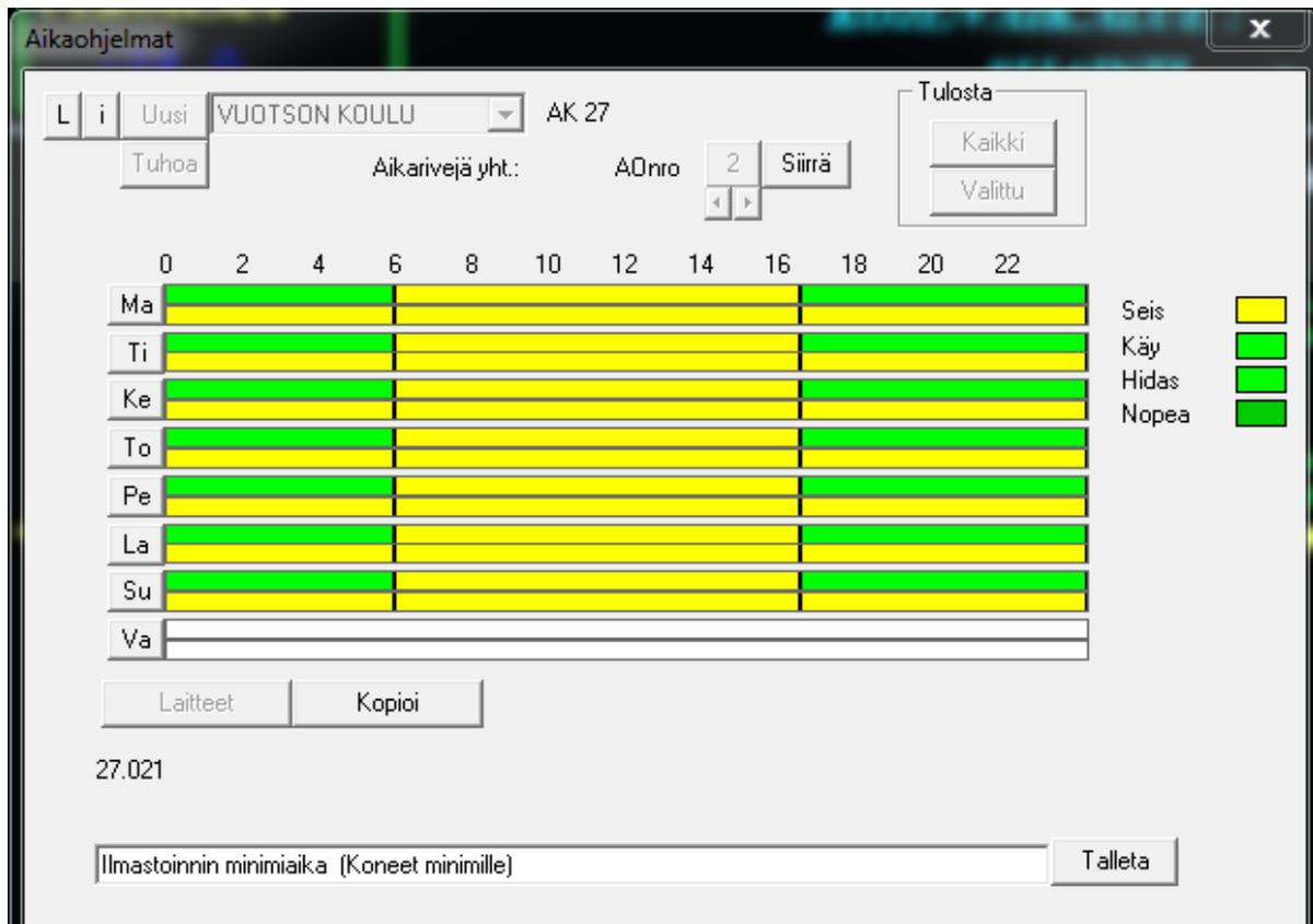
Figure 9: At night time the ventilation is at minimum power
